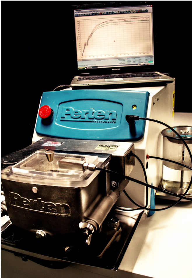
Perten Dough Lab conducting a farinogram.
