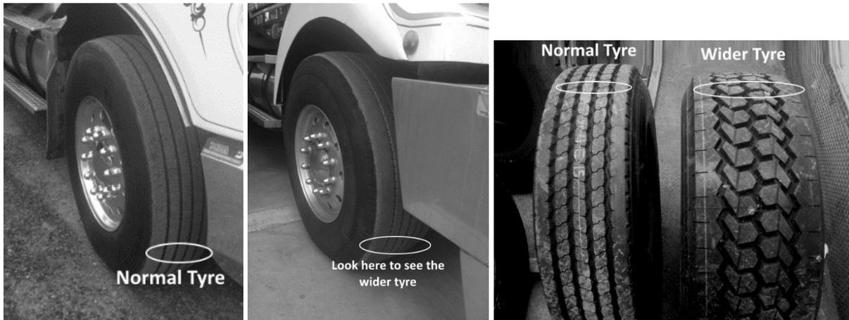
To physically confirm the tyre width, details are written on the tyre side wall. The first 3 digits should start with 375 or higher. For example, 375/90R22.5 indicates the tyre width is 375mm and is OK. Care must be taken when checking tyre side walls because it can be difficult for truck drivers to see pedestrians so close to the truck.
